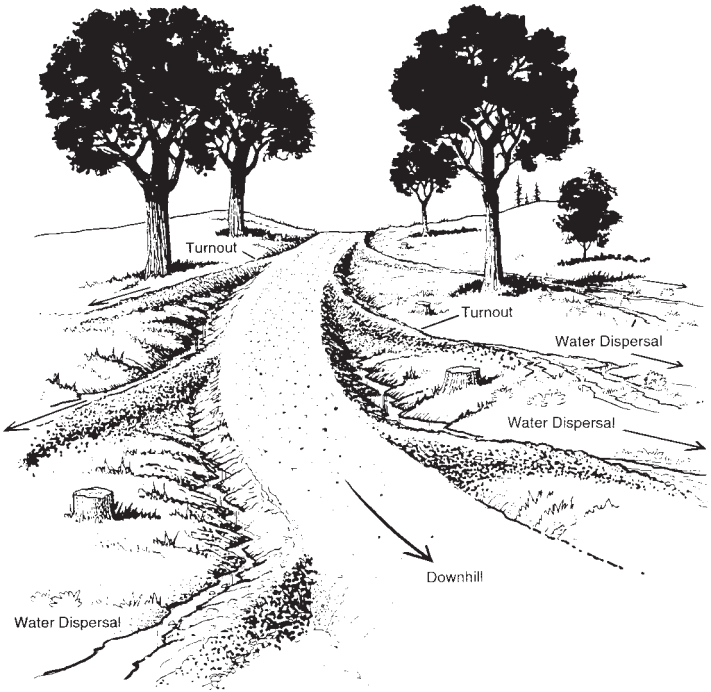
Figure 7. Installation and Design of Turnouts
